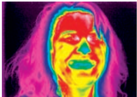
Figure 5-70. The nose of a person's face is often colder than other parts of the body due to less blood flow and more convective cooling.
