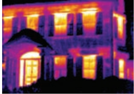
Figure 5-49. Areas of missing insulation show up as warm spots from the exterior of a building during cold weather.
