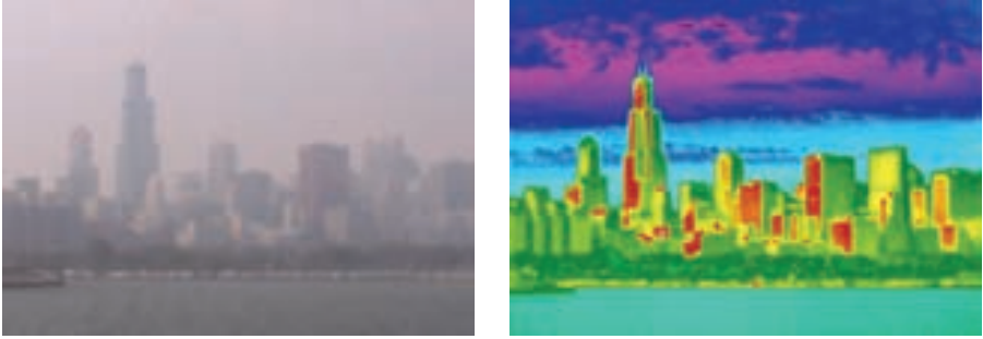
Figure 5-32. In the visible light photo, it is difficult to clearly see the details of the city skyline, or the sky, on a hazy, late-summer day. However, with thermal imaging, the details, as well as the different types of clouds in the sky, can be easily seen.
