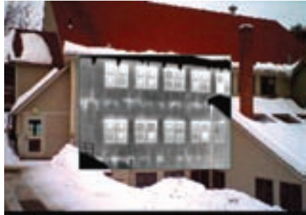
Figure 5-63. The many warm areas on the exterior front wall of a commercial building are associated with poorly installed fiberglass insulation.
