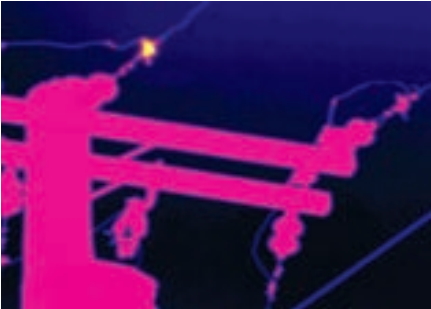
Figure 5-16. A high-resistance connection on a jumper (possibly due to corrosion) can have significant consequences if the load were to increase further.
