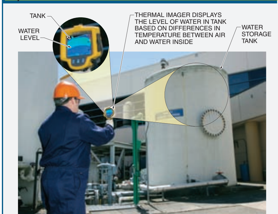
Figure 6-4. One of the most common applications for thermography is locating or confirming levels of material in vessels such as storage tanks and silos.
