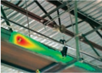
Figure 5-67. A belt rubbing against an overhead conveyor system tray creates a hot spot in the thermal signature. The belt became misaligned due to a nearby worn roller bearing. As a result, increased friction contributed to the overheating of a driver motor.
