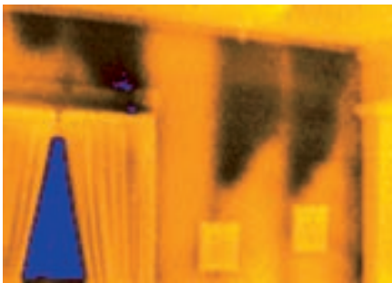
Figure 5-69. Poorly installed loose-fill insulation in an existing wall cavity can settle and not perform as well as it should.
