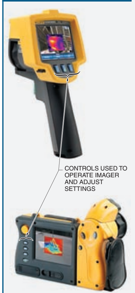
Figure 1-6. With controls, adjustments can be made to important variables such as temperature range, thermal span and level, and other settings.
